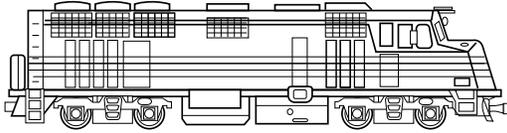
**BO-BO AMTRAK F40PH (1980):** The Bo-Bo is a diesel-electric passenger locomotive. This engine is ideal for handling passenger cars.
