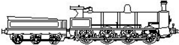
high-pressure cylinders and a single low-pressure cylinder between the frames. In various modifications, over 470 were built and the last was not withdrawn until 1964. They were found especially useful in the mountainous regions in and near Wales.
