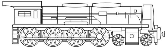
**4-6-2 A4 Class:** Possibly the most popularly known steam locomotive in Great Britain, this streamlined Pacific engine holds the world speed record for steam, 126 mph. Built from 1935 to 1938, they were not displaced from their role as express locomotives until the arrival of diesels in the 1960's. In the interim they powered the crack trains of the London & North Eastern, including "The Silver Jubilee" from London to Newcastle, the "Coronation", and the "West Riding Express".
