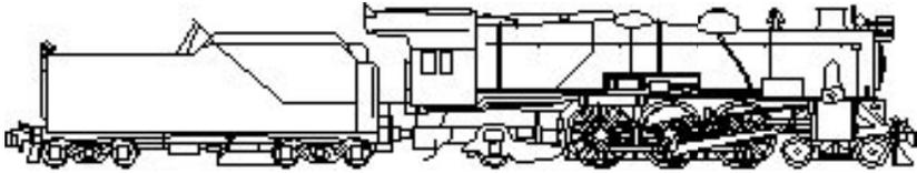
**4-6-2 Pacific:** Baldwin Locomotive Works claims the first Pacific type, delivered to New Zealand in 1901, although locomotives going back to 1889 had the wheel arrangement. Early into the 20th Century the Pacific became the preferred locomotive for almost all express passenger trains and many fast freights,
