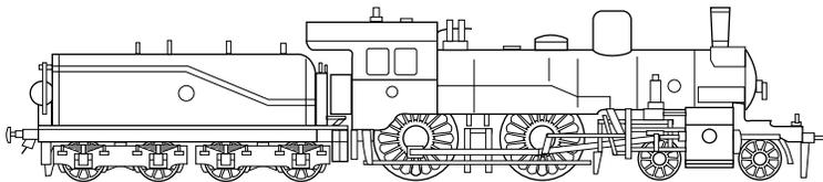
**4-4-0 CLASS S3 (1890):** A two-cylinder passenger locomotive. The S3 was one of the most successful passenger locomotives ever to run in Germany. Near the turn of the century over 1,000 of these locomotives were built.
