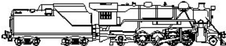
**2-8-2 Mikado:** The first 2-8-2s were built in 1897 for a railway in Japan, hence the name. The type was introduced in the United States in 1903, and it grew in popularity. It became the most common freight locomotive in the United States, partly because it was specified as an authorized design by the federal government
