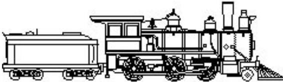
**2-6-0 Mogul:** The mogul engine type was developed to power heavy, fast freight trains that were too much for the American type which it bettered in tractive power by nearly 50%. The wheel arrangement had been tried as early as 1852, but a really successful mogul engine was not built until 1864. The mogul type was on its way to replacing the American as a national type, at least for freight service, but was itself replaced by the 2-8-0 before it was firmly established.
